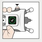
Place the tonometer at a 90 degrees angle on your face and take the measurement as previously instructed.
