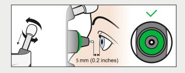
If the rings are not symmetrical, the probe does not point perpendicularly to the center of your eye. Correct the position of the tonometer. Keep both eyes open. Covering the eye not being tested may help you see the rings more clearly.
