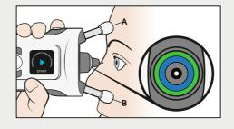
Before the measurement, adjust the forehead and cheek supports to the correct length. Start with the supports at the maximum length.
