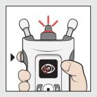
If an error occurs, the probe base flashes red. The display and sounds indicate the source of the error.
