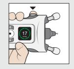
Place the tonometer at a 90 degrees angle on your face and take the measurement as previously instructed. After a successful measurement, press the Measure button (•) once and repeat the measurement on your other eye.
