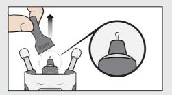
Drop the probe from the container to the probe applicator. Remove the probe applicator.
