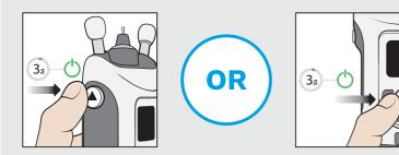
Press down () until you hear a beep. The text "Start" is shown on the display. Alternatively, press down • until you hear a beep. Then press • again to enter the measurement mode. The text "Start" is shown on the display.
