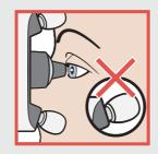
Before the measurement, adjust the forehead and cheek supports to the correct length. Start with the supports at the maximum length. Shorten the supports only two clicks at a time to prevent the tonometer from getting too close to your eye.
