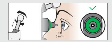
If the rings are not symmetrical, the probe does not point perpendicularly to the center of your eye. Correct the position of the tonometer. Keep both eyes open. Covering the eye not being tested may help you see the rings more clearly. Shorten the supports by rotating them clockwise two clicks at a time until you only see a symmetrical green ring. The tonometer is now at the correct distance from your eye.
