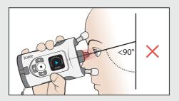
The forehead support A rests on your forehead and the cheek support B rests on your cheek. Look straight ahead and the tonometer is at a 90-degree angle to your face. The probe is about 5 mm from your eye and points perpendicularly to the center of your eye. If you see a red light in the probe base, the tonometer is tilted too much downwards. You should straighten your posture and lift your chin.
